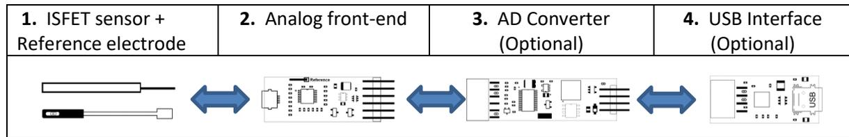
➔ Modules 1 and 2 are always needed to conduct pH measurements with the test kit. Modules 3 and 4 are optional.
