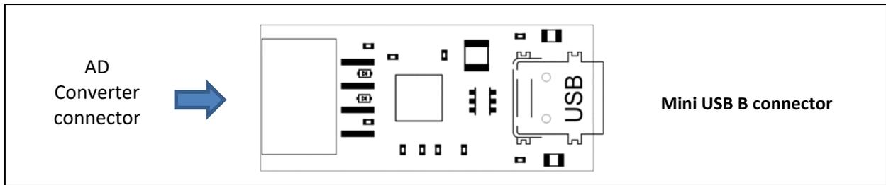
The USB interface provides a USB 1.1 or 2.0 connection to a computer (note the USB interface is not USB 3.0 compatible). It is possible to connect multiple USB interface modules to one PC, up to the current limit of your USB ports.
